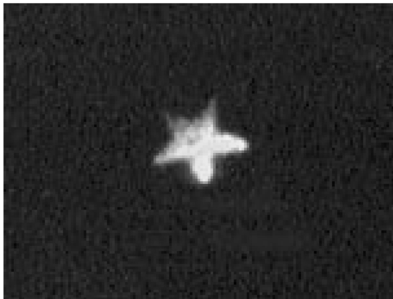
FIGURE 4 EL output pattern from the light transducer composed of Me-PTC/PC-Z film and EL layer. The input light through a star-shaped mask was illuminated from the other side.
